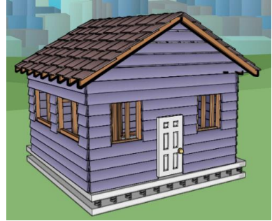
House with a base isolation foundation
