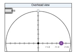
2. The speed of rotation is described by **angular velocity** ( $\omega$ ), which is measured in radians per second. There are  $2\pi$  radians (6.28 radians) in a circle.
